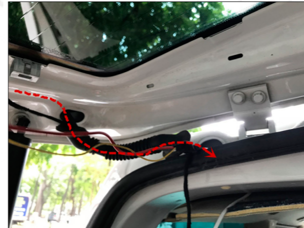
15. Thread the harness from the waterproof bellows to the car body.
