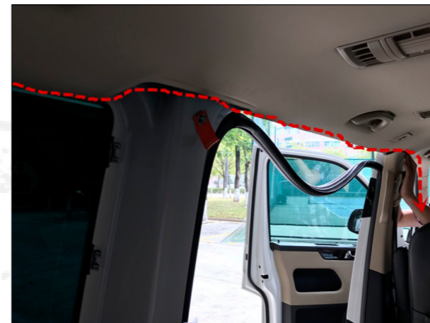
17. Route the power and signal lines to the main driver's seat.
