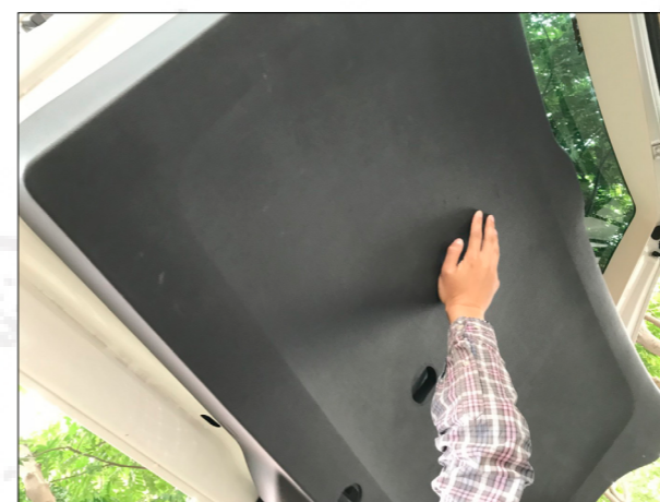
5. Remove the tailgate cover.
