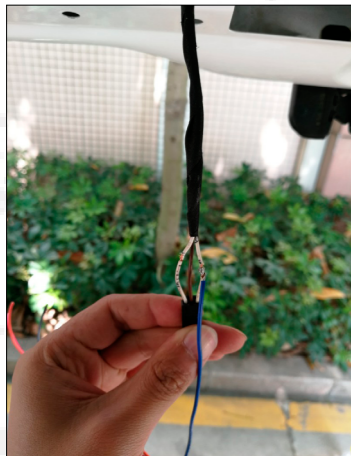
11. Unplug the white wire on the right side of the original car lock signal plug and connect the blue wire of our lock switch cable.
