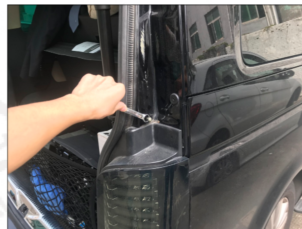
7. Remove the original car body ball head and install our car body ball head.
