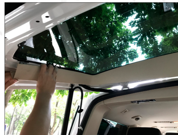
3. Remove the tailgate lone plaque.
