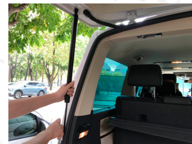
6. Remove the original car poles.
