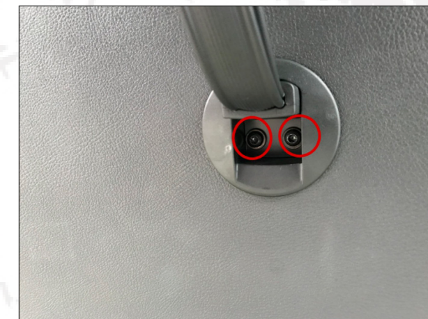
4. Remove the two fixing screws of the tailgate trim.
